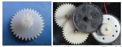
Figure 2: Gear with lower & upper part having different no. of teeth Figure 3: Gear Train
